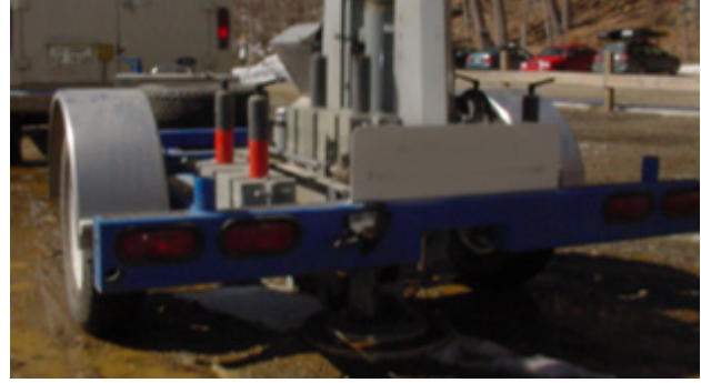
b. Close up of the back of the trailer holding the falling weight deflectometer.
