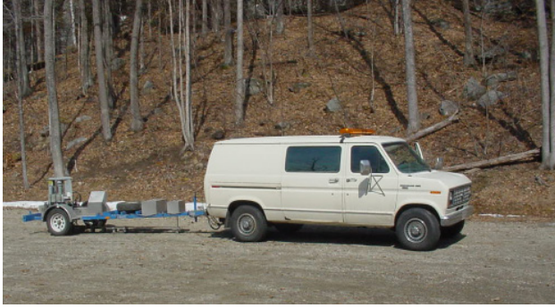
a. Van pulling a trailer that contains the falling weight deflectometer on a gravel lot.
